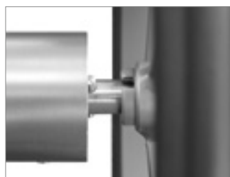
Drive wheel arrested in free-wheel function
