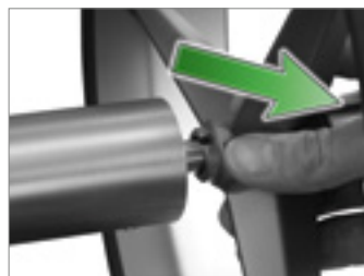
Removing and attaching the drive wheels
